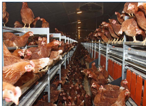
Aviary systems utilise the vertical space within a facility to allow better use of the facility and to provide environmental enrichments to increase bird welfare.
