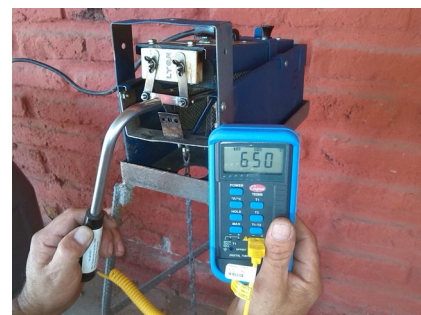
Pyrometer indicating proper blade temperature of 650°C.
